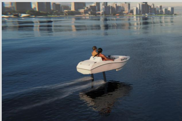
These hydrofoils are underwater wings autonomously controlled by computer, allowing the boat to lift and glide above the water.
